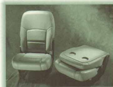
The lightweight modular rear seats fold flat when not in use. The seat backs convert into convenient tray tables with built-in cupholders.
